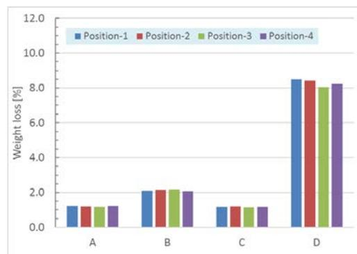
Fig. 1 Impact of the sample position on the weight loss by the plasma exposure.
