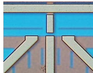
Figure 1: Chip micrograph of open pattern.
