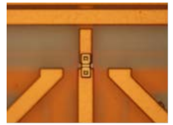
Figure 2: Chip micrograph of short pattern (after FIB process).
