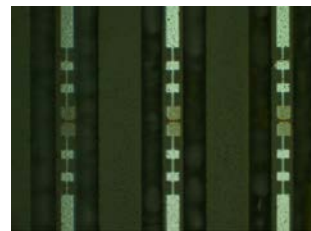
Fig. 1: 1.9 THz band horn/waveguide type superconducting HEB chips diced with the DISCO's dicing blade. The chip thickness is 18 μm. The chip width is 36 μm.
