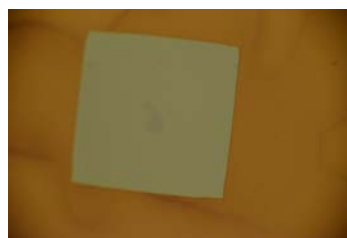
Fig. 1 Optical microscope image of 1 mm×1 mm dielectric membrane
