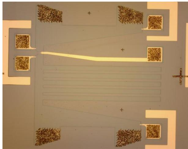
Fig. 1 Optical microscope image of a sample. Evaporated gold metals function as metal gate electrodes.
