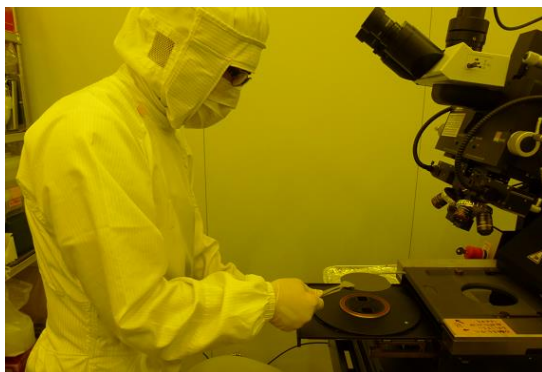
Fig. 1 Photomask alignment process.
