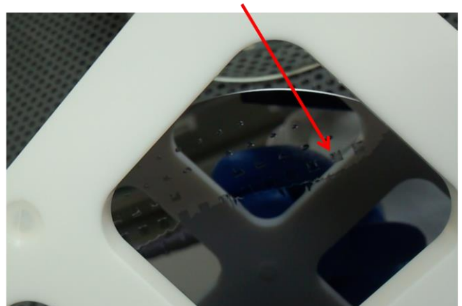
Fig. 1 Wafer image after removing photolitho resist
