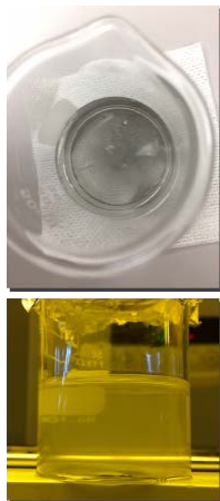
Fig.1. Ga sample in ethanol, which was ultrasonically cleaned at 50°C.
