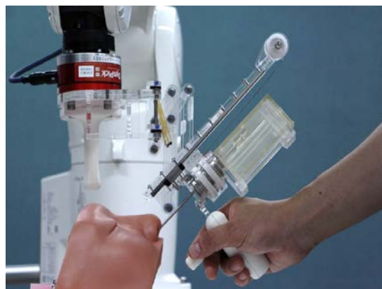
Fig. 1 Experiment of usability of user interface in a nasal model for surgical training.
