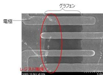
Figure 1 Scanning electron microscope image of graphene patterned by photolithography.
