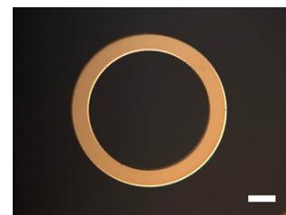
Fig. 2 Optical microscopy image of metal ring pattern fabricated by photolithography with lift-off process. Scale bar is 20  $\mu$ m.
