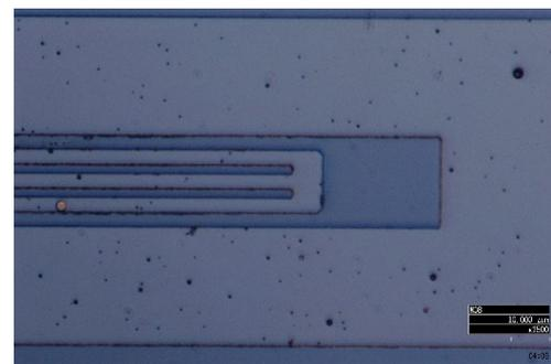
Fig. 2 Image of the surface with particles.
