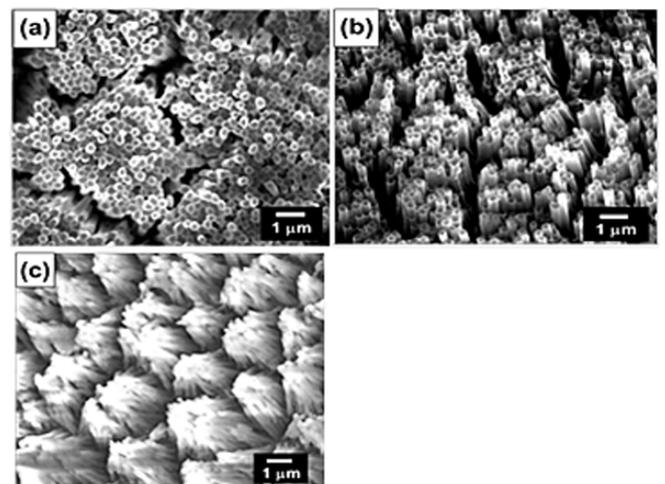
Fig. 1 SEM images of (a) poly(HEMA-Br-co-MCMA)-based polymer pillar film, (b) polymer pillar film after photoirradiation, and (c) the polyTFEMA-grafted polymer pillar film from.
