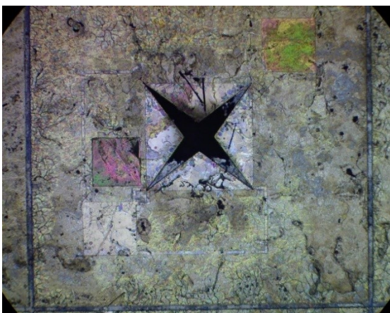
Fig. 1 Device image of prototype piezoelectric MEMS sensor.
