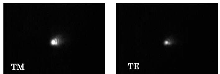
Fig.2 Near field images for the fabricated Si slot waveguide for TE and TM polarized light.
