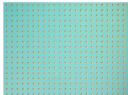
Fig. 1 Top-view optical microscope image of SU-8 pattern. The diameter and pitch of micropillar are 10 and 50  $\mu\text{m}$ , respectively.
