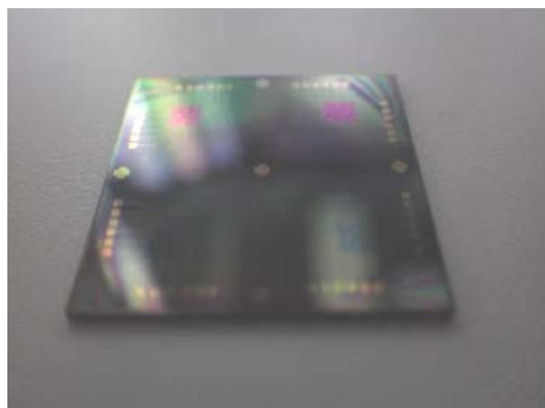
Fig. 1 Self-alignment substrate treated with hydrophobic material
