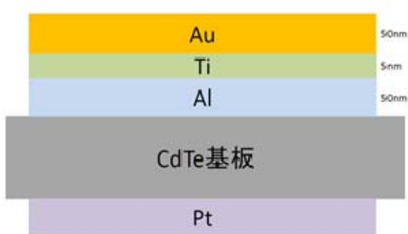
Fig.1: Structure of CdTe detector
