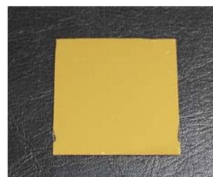
Fig. 1 Photograph of gold thin film formed on polystyrene substrate.
