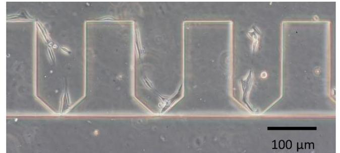
Fig.1 Trapped cells in the microfluidic device
