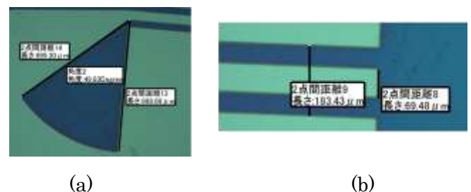
Fig. 2 Measurement of the Fin-line (microscope)
