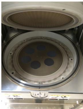
Fig.1 Φ2-inch GaAs wafer on the stage.
