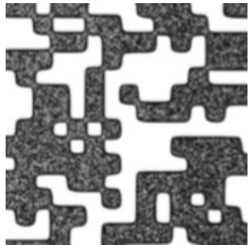
Fig. 1. Image of the mask pattern captured by a laser microscope.
