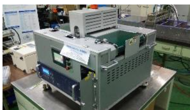
Fig.2 RF-type atmospheric pressure plasma apparatus
