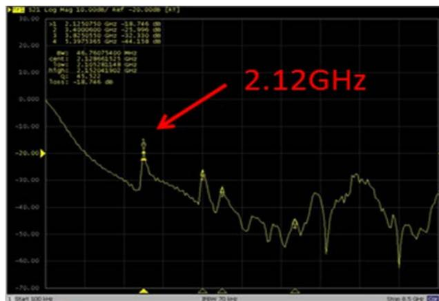
Fig. 2 Resonance characteristic of fabricated MEMS resonator
