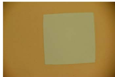
Fig. Optical microscope image of 300 \mu\text{m} \times 300 \mu\text{m} dielectric membrane
