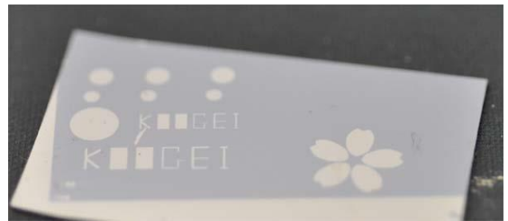
Fig. 2 Si substrate after DeepRIE process.
