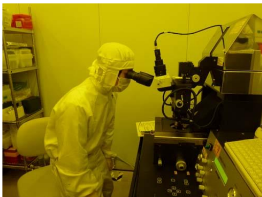
Fig. 1 Photomask alignment process.
