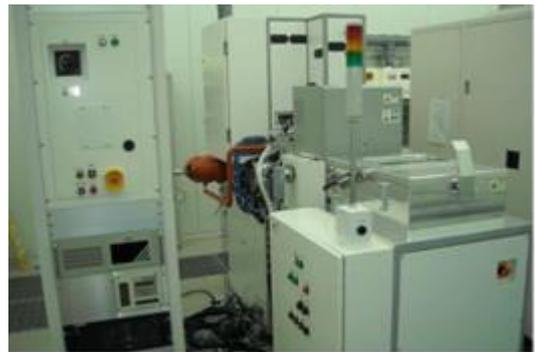
Fig. 1 Plasma-enhanced chemical vapor deposition system.
