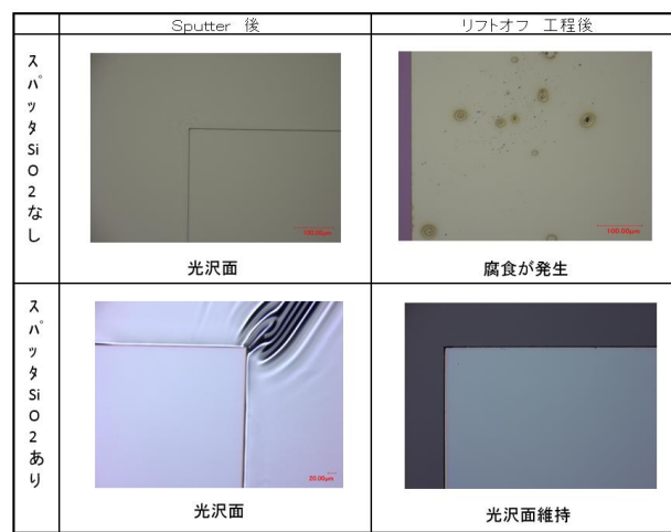
Fig. 1 Microscopic image of Fe-Si-B surface with and without SiO 2 respectively
