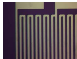
Fig. 1 Al pattern formed using MX-1204 (linewidth:7um)
