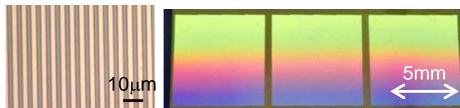
Fig. 2: (a)Patterning result of 4μm-pitch grating. (b)Photo of the fabricated gold grating.
