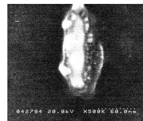
Figure 2. A SEM image of lifted off nanoparticle pattern
