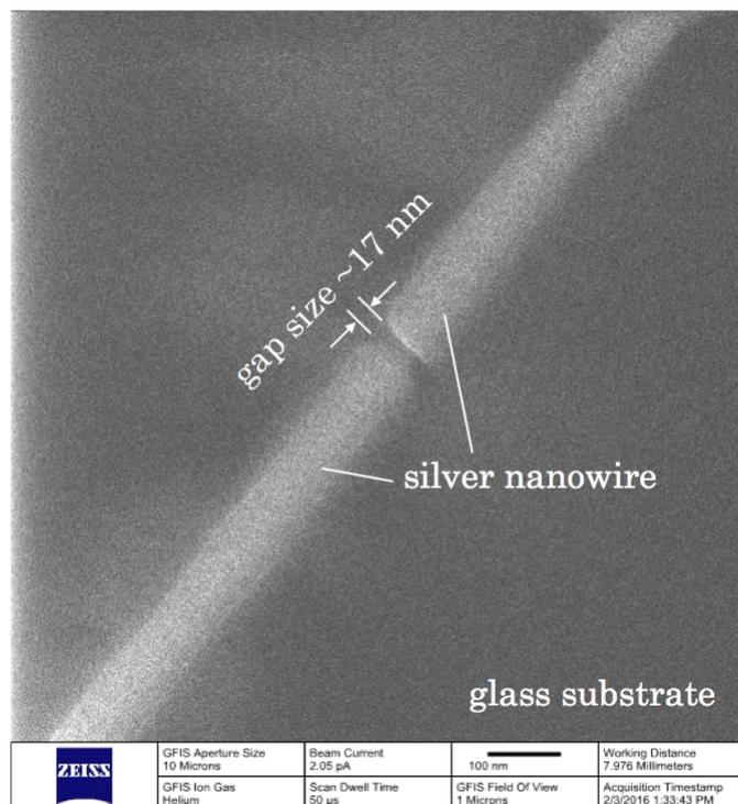
Fig. 1 A scanning ion-beam microscope image of a silver nanowire cut with He-ion beam.
