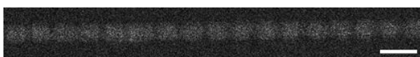
Fig.1 Nanofiber with the grating structure fabricated by helium ion beam. Scale bar indicates 500 nm.
