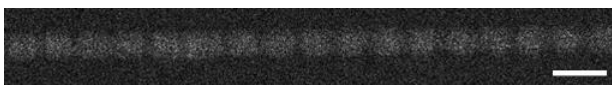
Fig.4 Nanofiber with the grating structure fabricated by helium ion beam. Scale bar indicates 500 nm.
