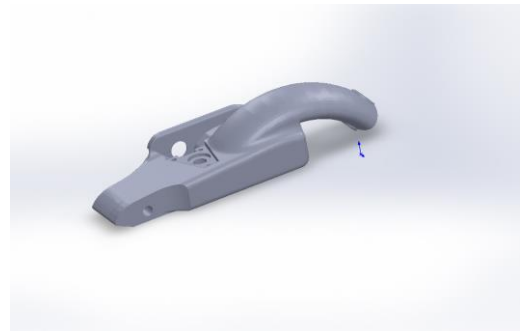
Fig. 2 Designed Palm Part of Long Finger.
