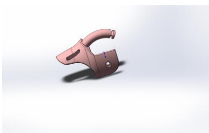
Fig. 1 Designed Fingertip Part of Little Finger.
