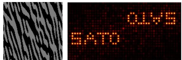
Fig.1. Calculated phase pattern for a diffractive optical element and simulated diffractive pattern.
