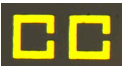
Fig. 1 Microscopic image of split ring resonator.
