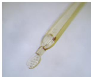
Fig.2 Device with protein crystals.
