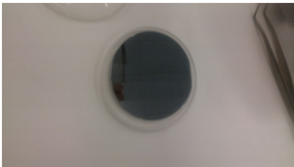
Fig. 1 Silicon wafer divided into chip by dicing.
