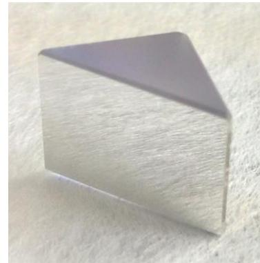
Figure 1 Experimental Sample. ~50 nm silver film were deposited on the glass prism.
