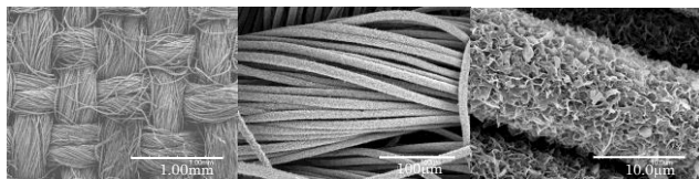
Fig. 1 SEM images of MnO_2 film deposited on a carbon cloth electrode.
