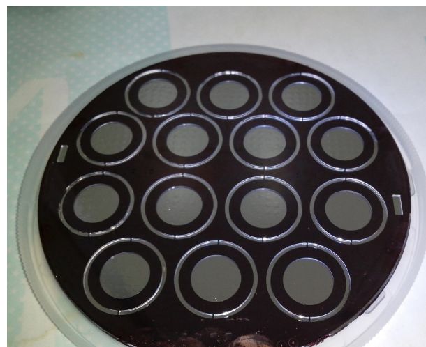
Fig. 2 Etched Si wafer (4 inch) : its etching is stopped with Ni sputter membrane (400 \mu\text{m} depth).
