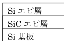
Fig. 2 Si epitaxial growth on SiC layer on Si substrate.
