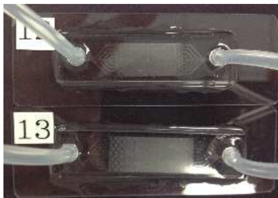
Fig. 1 Micro fluidic devices having the cross section patterns of virus filters.
