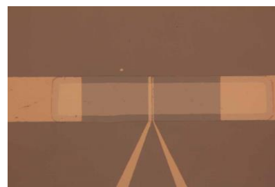
Fig.3. Photograph of a fabricated sample for characterizing spin injection and detection through a \gamma' -Fe 4 N/GaN Schottky barrier.
