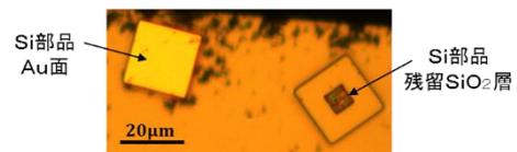
Fig.2 Microscopic image of manufactured silicon components.
