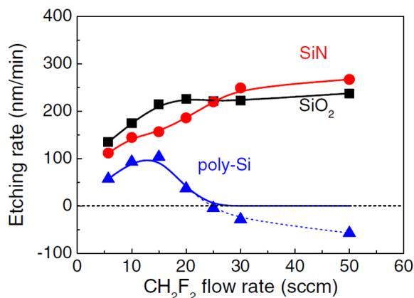
Fig. 1 Etching rate as a function of a flow rate of CH<sub>2</sub>F<sub>2</sub>.
