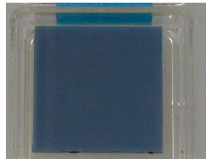
Fig.1 A photograph of a thin film of microcrystalline Si deposited with the radical injection plasma source.
