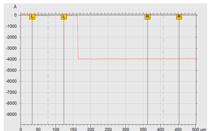
Fig. 1. Step profile of dry-etched sample. Etching time was 10 min.
